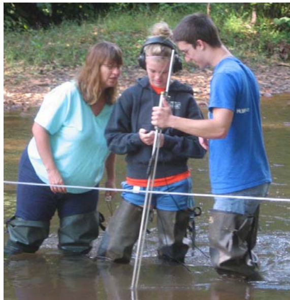
Shikellamy teacher, Sheila Furr, and two students performing flow rate measurement of Shamokin Creek.
