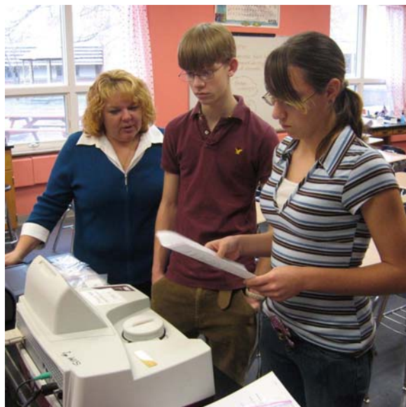
Yvonne Monahan's Shikellamy High School students attempt to determine the brand of plastic wrap found at the crime scene using an FTIR.
