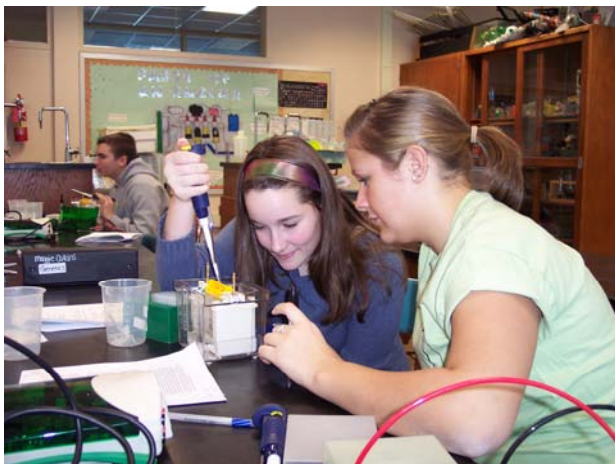
Central Columbia students load a vertical polyacrylamide gel to analyze PCR products in the GMO Investigator lab.
