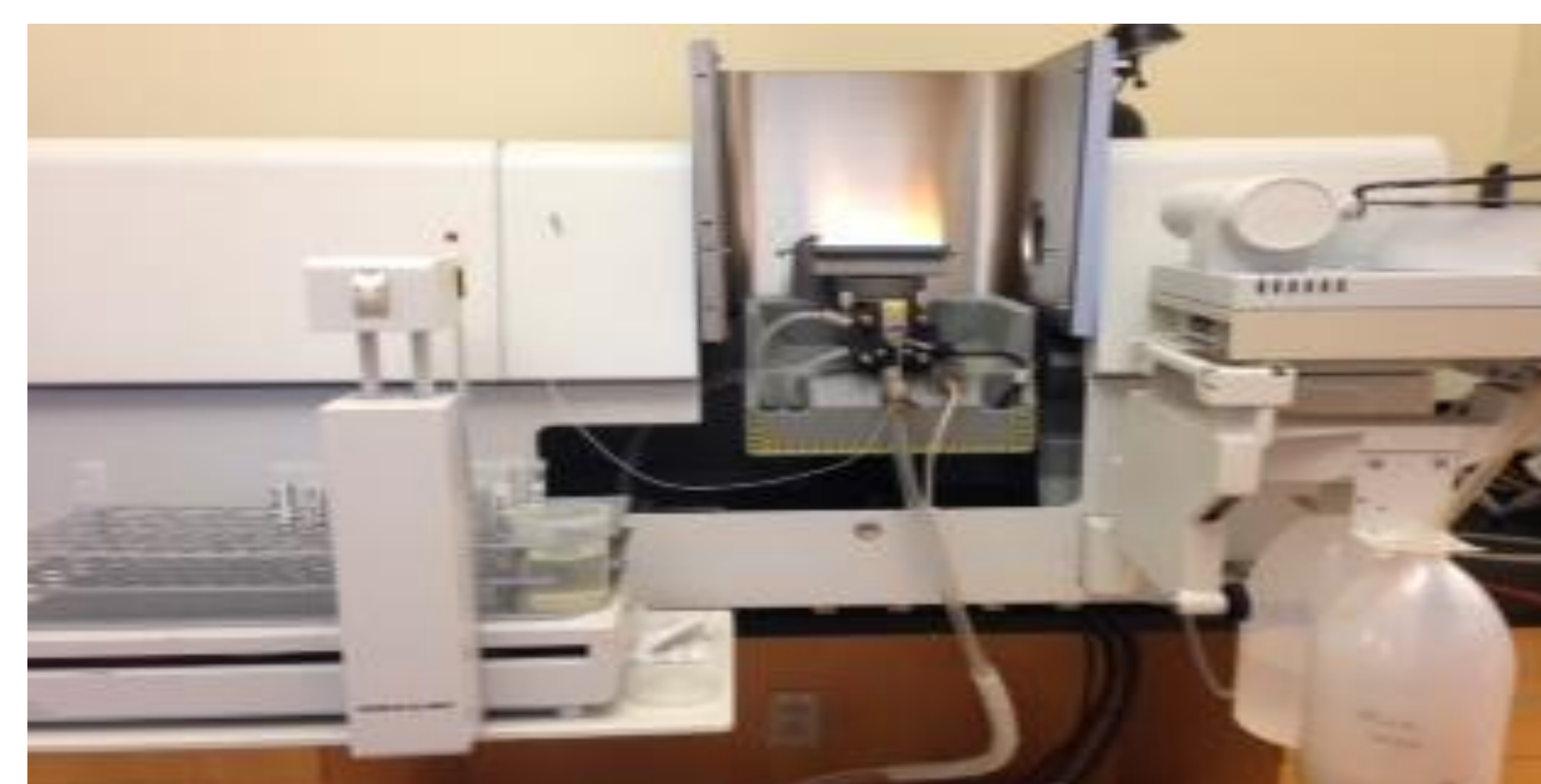
Figure 2. Flame atomization using the Perkin Elmer AAnalyst 800 Atomic Absorption Spectrometer for a sample of magnesium, which yielded an orange flame.
