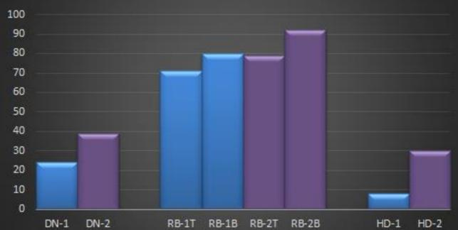
Figure 2: Percent Ephemeroptera, Plecoptera, and Trichoptera (%EPT) for three collection methods, D-Nets (DN), Rock Baskets (RB), and Hester-Dendy Samplers (HD). On top of cinder block (T), Bottom/on Substrate (B). Site 1(1) is blue, and Site 2 (2) is purple. %EPT describes the observed pollution sensitive taxa.
