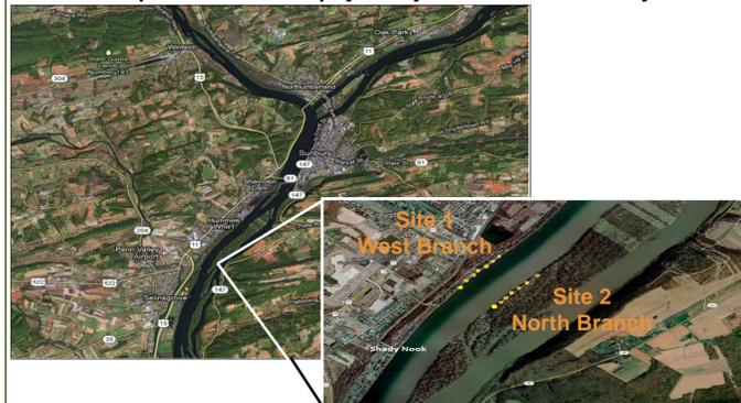
Figure 1: Aerial image of Byers Island and site locations along the west channel of the upper main stem of the Susquehanna River. The active methods were employed in six locations at each site, 100m apart and above the passive sites. The passive methods were used in the most southern location on either side.
