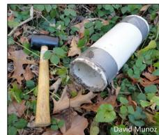
Figure 3. PVC soil sampler
